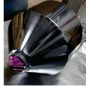
Figure 1: The horizontal cavity spacer has a biconic shape with specific cut angles to reduce the sensitivity to accelerometric noise.
